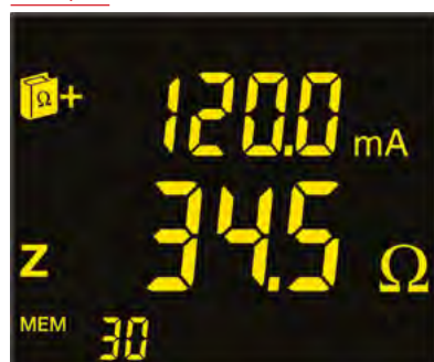
Screen 1: Impedance and leakage current
