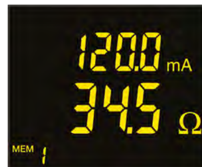
Standard mode: Impedance and leakage current
